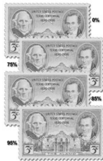
Figure 7. Compressing JPEG images saves storage space. There is an inverse relationship to image quality, the degradation of which becomes particularly noticeable at high levels of compression.
